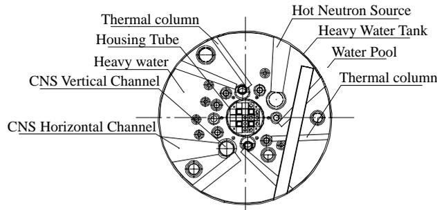
Fig. 1. The core layout of the CARR.
